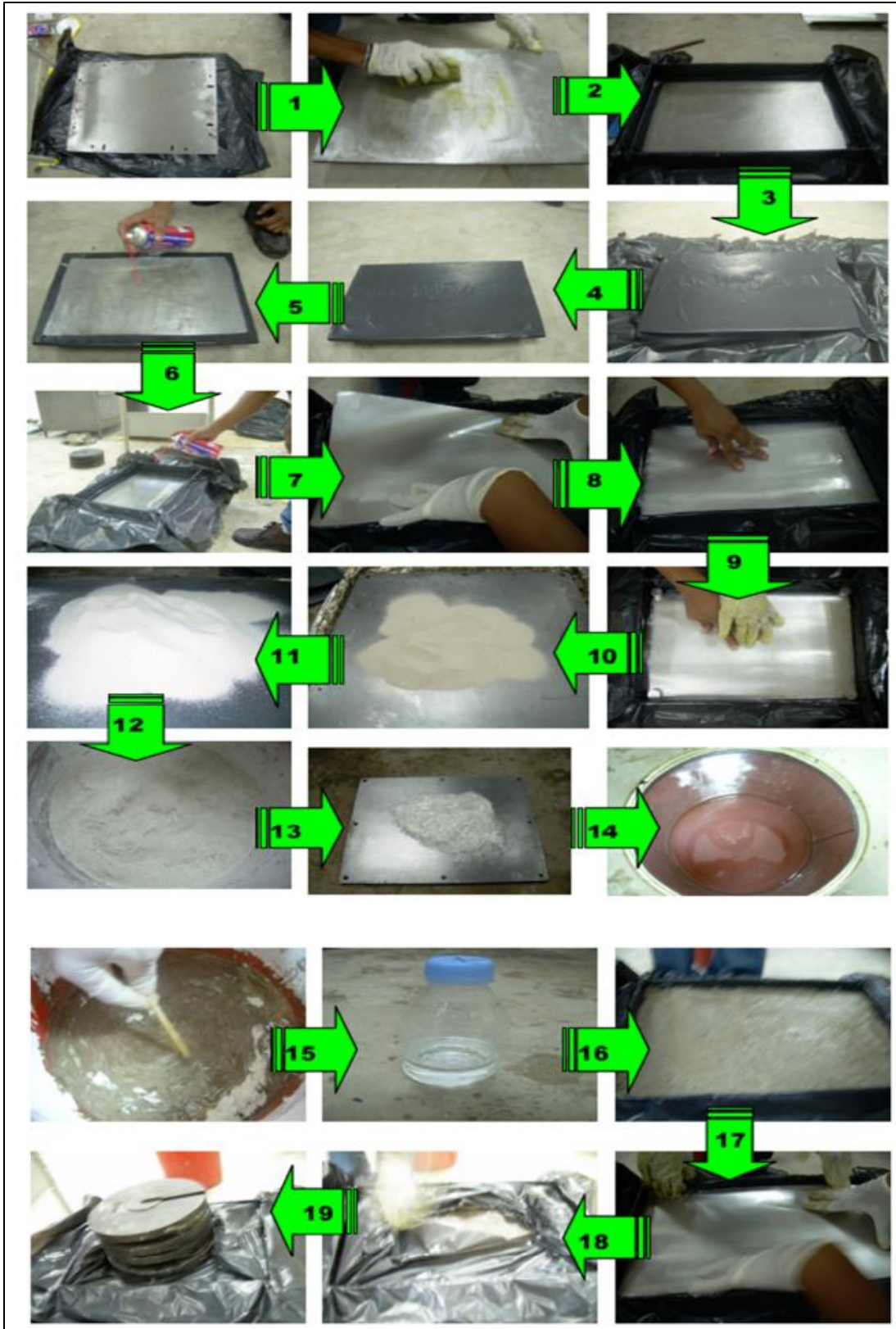
Figure 4 The Process of Polymer Mixed Concrete Preparation
